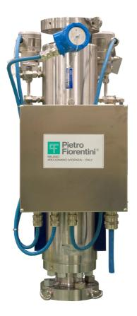
The flow rates of oil, water and gas are calculated based on the measurements of the fluid dielectric properties, of the differential pressure across the venturi inlet. No separating devices, mixers or bypass lines are needed.
