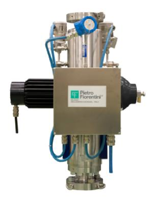
The flow rates of oil, water and gas are calculated based on the measurements of the fluid dielectric properties, of the differential pressure across the venturi inlet and of the density through the gamma ray detection. No separating devices, mixers or by-pass lines are needed.
