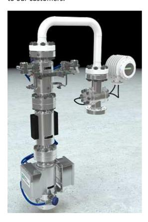
The flow rates of oil, water and gas are calculated based on the measurements of the fluid dielectric properties and of the differential pressure across the venturi inlet..
